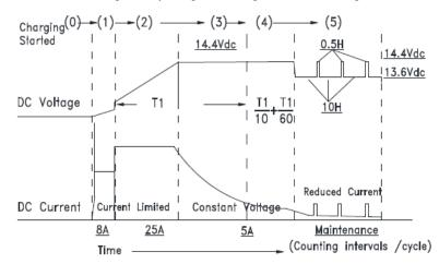
Total Charge Time: 12 minutes + T1 + T1/10 + T1/60 Time T1 = Time of Step 2 + Step 3 (start after soft start and end at charger output decrease at 5A ) T1 to different by battery capacity & battery start charge level
